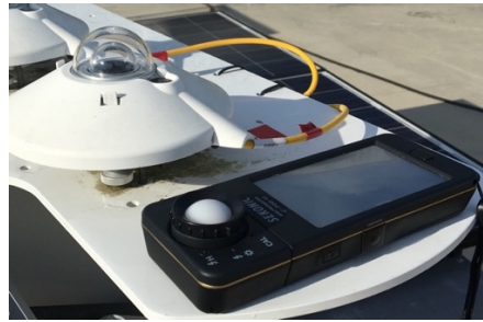
Fig. 7. Solar irradiance and illuminance data collection setup
