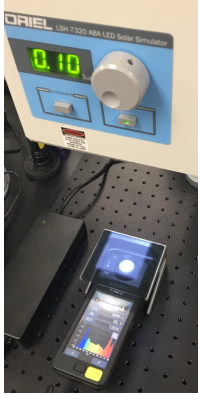
Fig. 6. MiniSol solar simulator, ND filter, stand, and light meter
