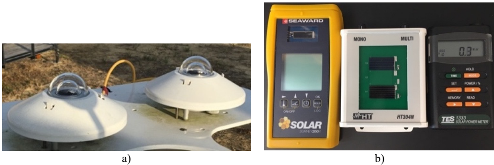
Fig. 2. Solar irradiance measurement devices: a) pyranometers and b) silicon devices
